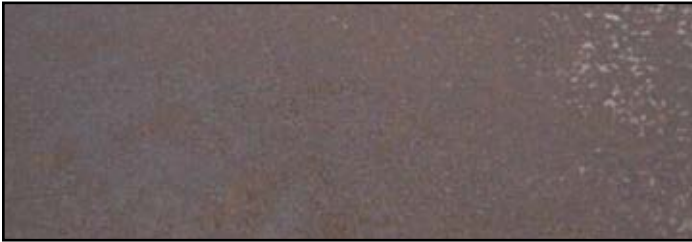
Figure 2. Salt coated steel sample after 500 cycles.
