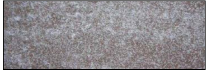
Figure 3. Salt coated steel sample with CONDENSTOP after 500 cycles.
